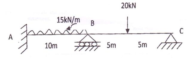
Q8) Analyze the continuous beam loaded and supported as shown in figure, if support B sinks by 10mm. Use stiffness matrix method. Take EI= 6000 kNm<sup>2</sup> [16]
